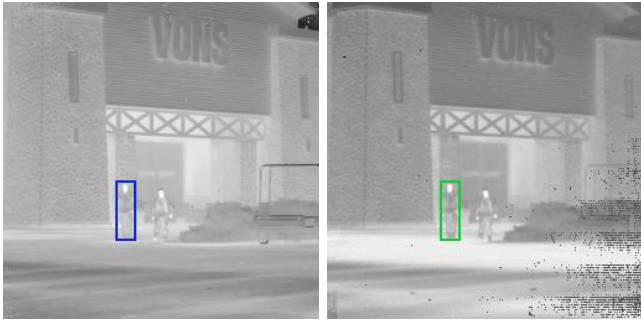
Fig. 2. Typical MWIR/LWIR frame pair acquired with the DBIR sensor of Fig. 1, cropped to a 240 \times 240 pixel 1:1 aspect ratio. The 8\text{--}12\text{ }\mu\text{m} longwave band is shown on the left, while the 3\text{--}5\text{ }\mu\text{m} midwave band is shown on the right where the swath of damaged pixels is evident. Ground truth bounding boxes (blue and green) are added for one object of interest.
