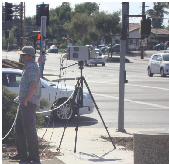
Fig. 1. Experimental dual-band MWIR/LWIR sensor deployed for field tests to acquire DBIR video sequences in Santa Barbara, CA.
