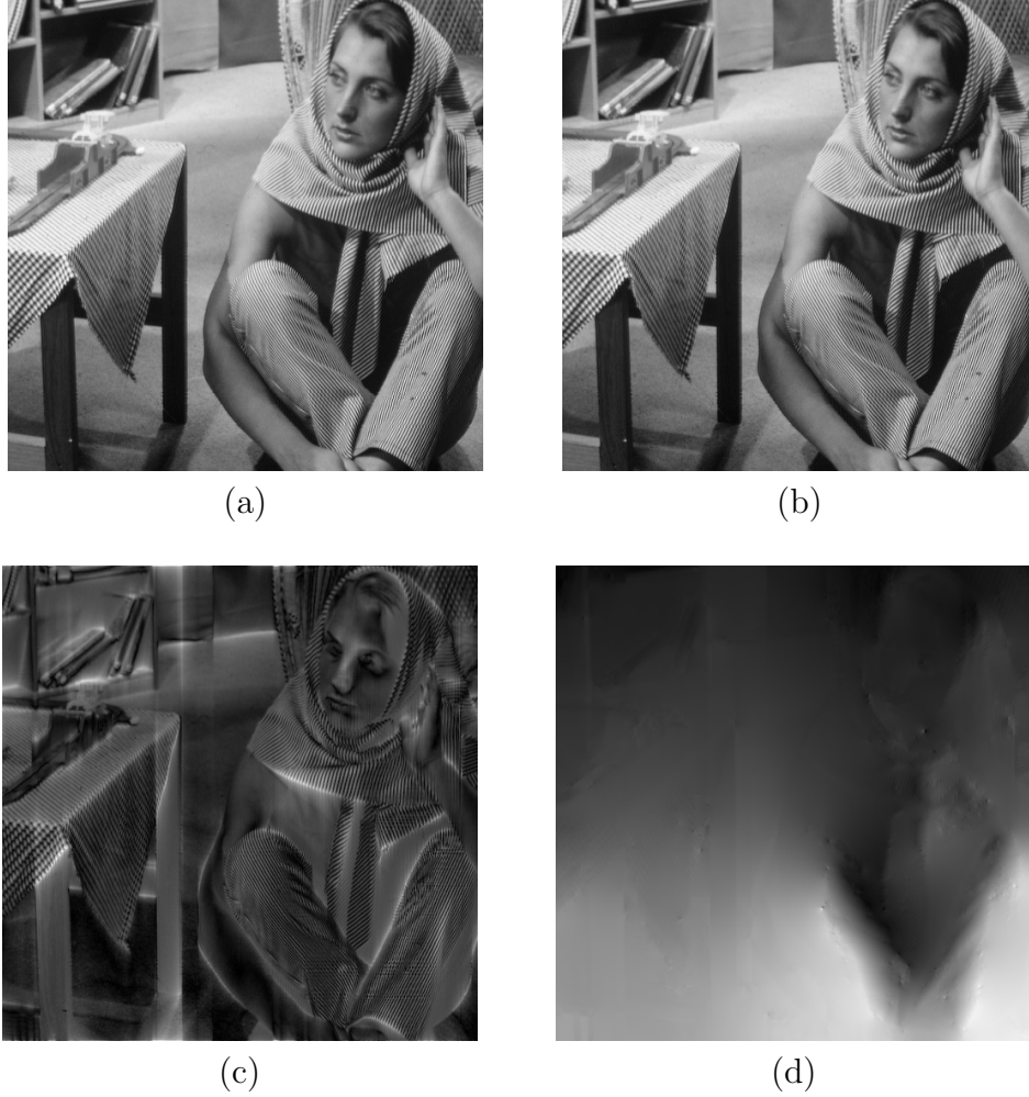
Figure 5.1: Single component AM-FM representation of the barbara image. (a) Original barbara image. (b) Reconstructed barbara image. (c) Computed AM function. (d) Computed phase function.
