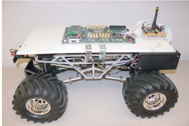
Fig. 4 Prototype mobile robot testbed with Virtex II pro reconfigurable platform
