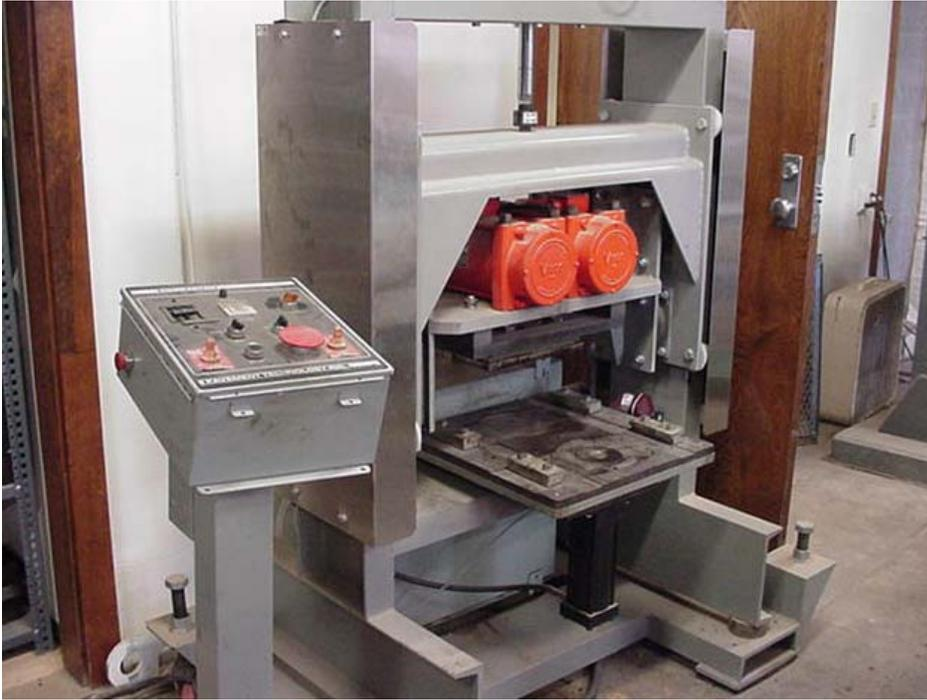
Fig. 1. Asphalt Vibratory Compactor
