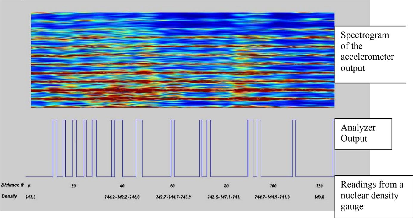
Fig. 6 Use of Analyzer to determine compaction in the field.
