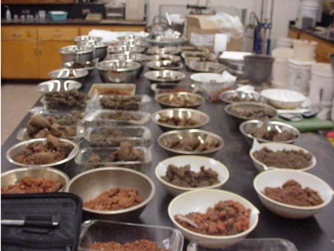
Fig. 11 Drying out the bulk samples prior to processing
