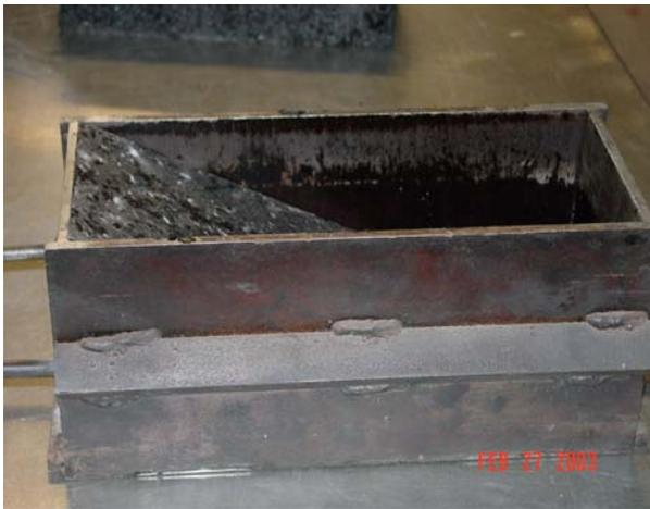
Fig. 2 Mold for compacting the mix
