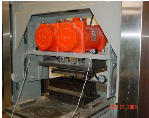
Fig. 3 Accelerometers mounted on the frame of the AVC to measure the vibrations of the compaction head
